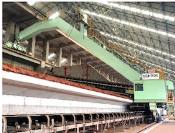
SCHADE Semi-Portal Reclaimer in operation at Baosteel (photo SCHADE)
